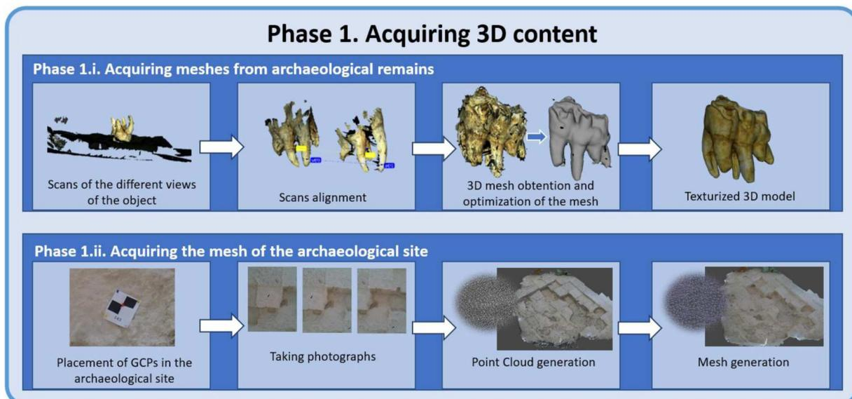
**Figure 4.** Phase 1. Acquiring and generating all the 3D content of the archaeological site.
