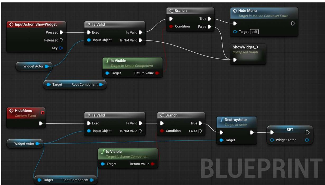
Figure 16. Part of the logic developed by Just2devs to show and hide a floating menu with a constant position and orientation relative to the user’s view, invoked or hidden with the A button of the Oculus Rift gamepad.
